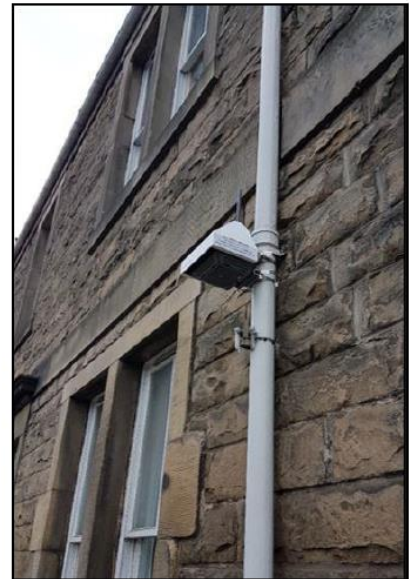
Appin Crescent West AQMesh Sensor (co-located with triplicate diffusion tubes Appin Crescent 6A, B, C)
