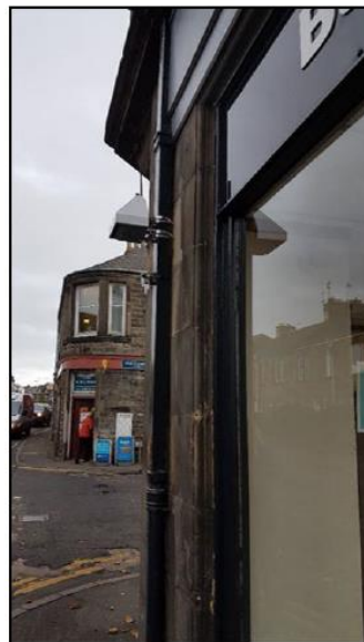
Appin Crescent East AQMesh Sensor (co-located with triplicate diffusion tubes Appin Crescent 5A, B, C)
