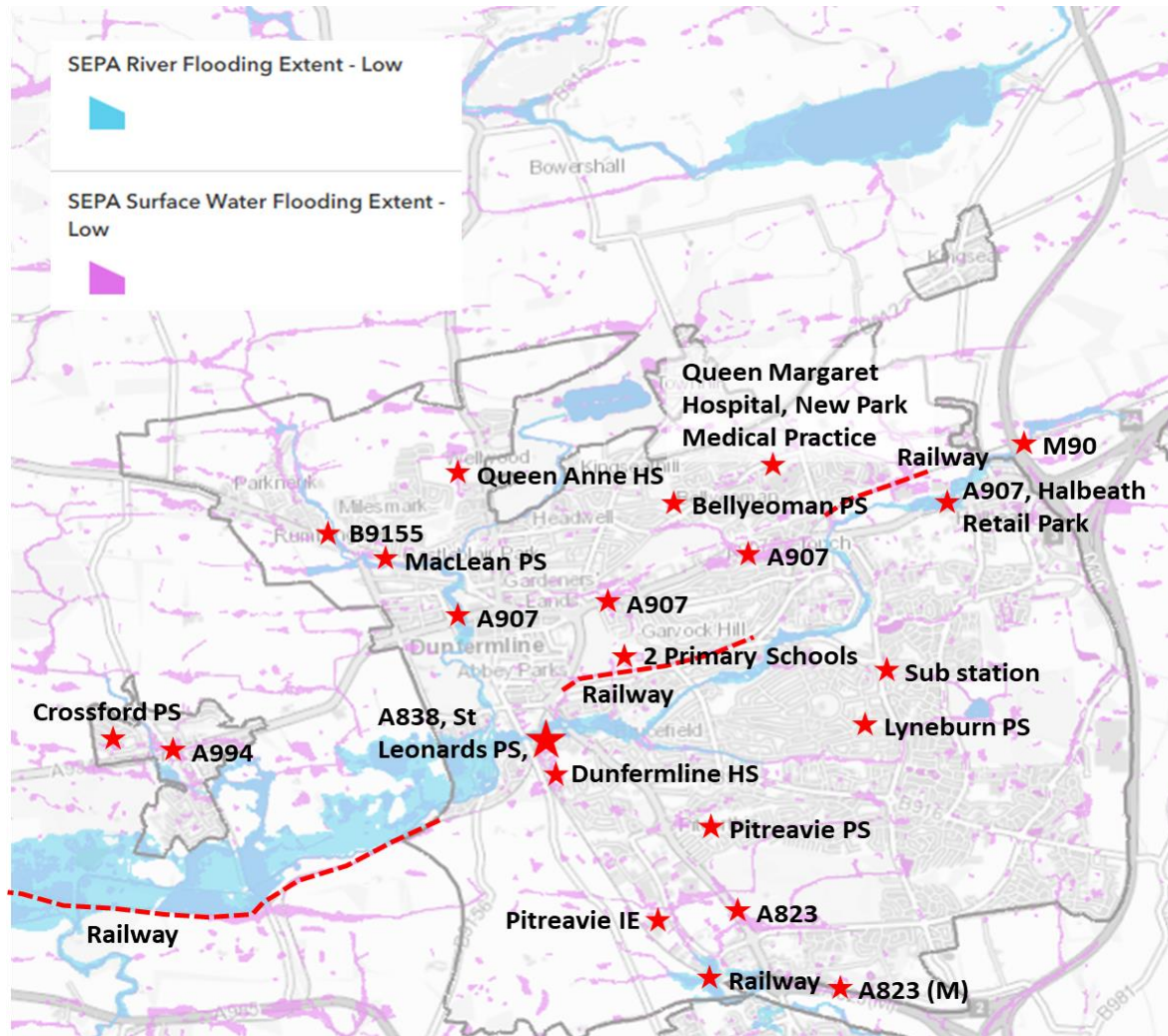
Figure 5.6 Plan showing key assets predicted to be at risk of flooding in the City of Dunfermline locality. This map was created by visually comparing: Fife Council data on schools, healthcare facilities and key employment areas (see Local Living and 20 minute neighbourhood interactive map ) and Mastermap and OS Base mapping with SEPA flood maps
