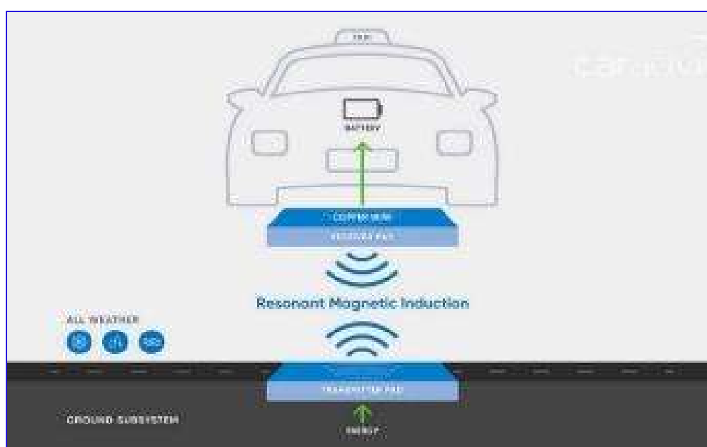
Figure D-1. Induction Charging
